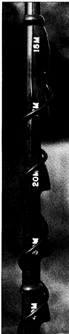
Close-up of the Outbacker JR8 antenna showing a few of its band taps and the "Wander Lead" band-changing wire.
